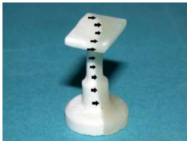
Fig. 10 – Example of casting with variable section channel and horizontal plate. The black arrows show the limit between the two materials. There are no evident areas of high turbulence
