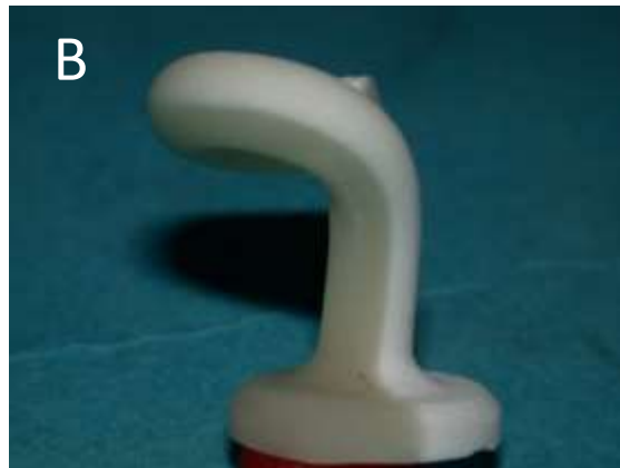
Fig. 8 (A, B) – Spiral channel after casting
