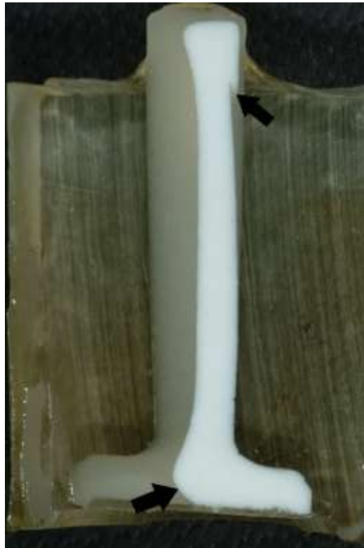
Fig. 15 – The median section of the straight pin shows a good conservation of the laminar motion of the materials during casting procedure (black arrows)
