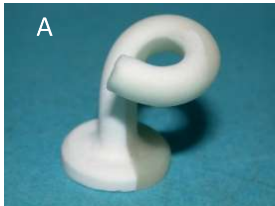
Fig. 7 – Channel with variable section after casting
