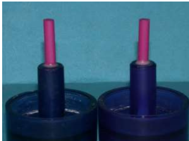
Fig. 1 – Straight pouring channels
