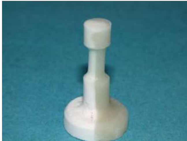
Fig. 7 – Channel with variable section after casting
